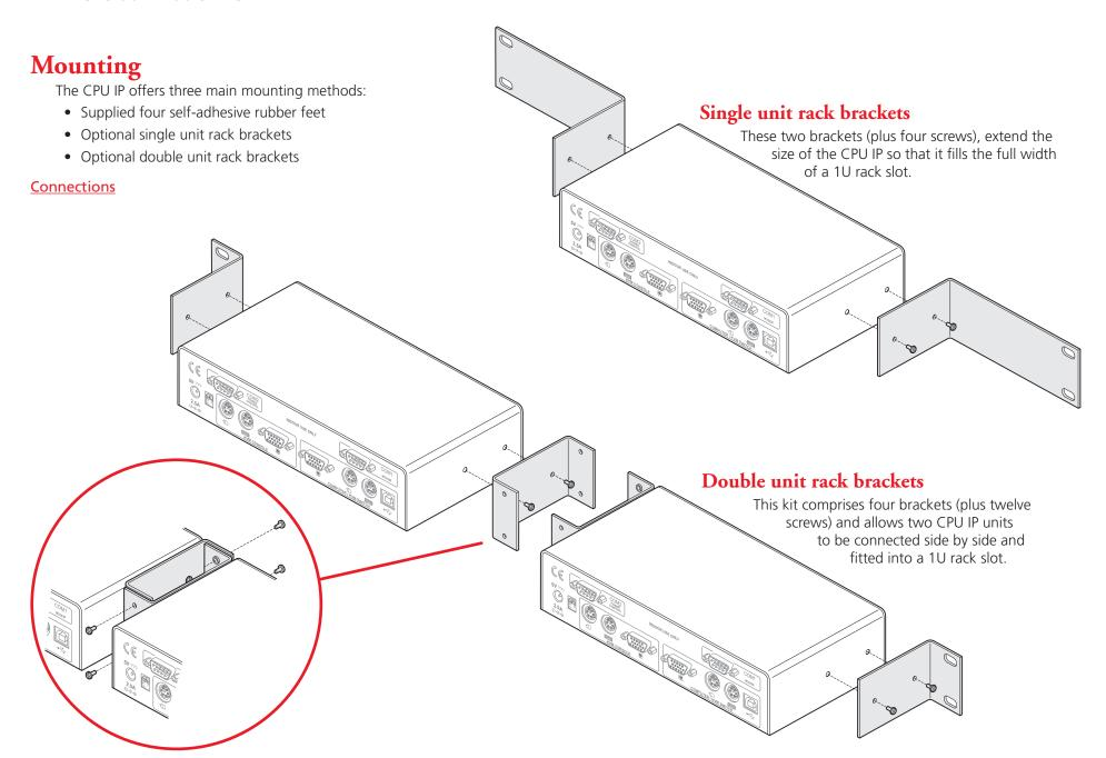
Installation of the CPU IP involves a number of basic connections to some or all of the following items:
